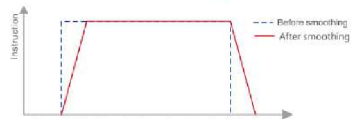
Figure A: When the controller sends a step signal of instruction, the stepper drive automatically smooth to a trapezoidal signal.
